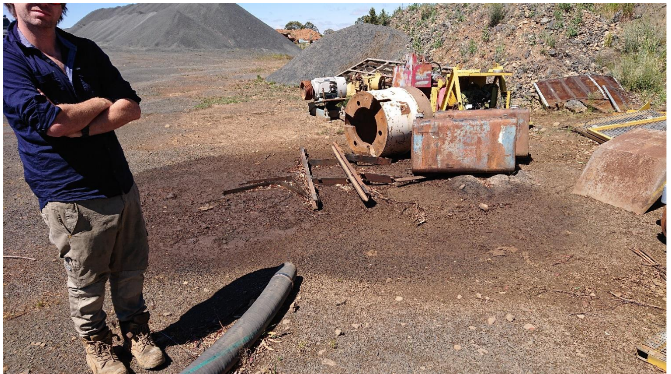
Photo # 6 - Oil seepage from derelict Equipment
